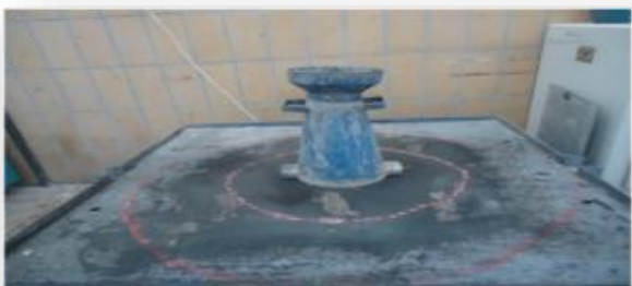
Figure 4: Cone apparatus prepared for slump flow test
