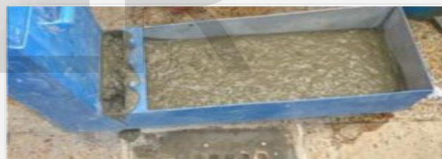
Figure 6: Test carried out in L-Box
