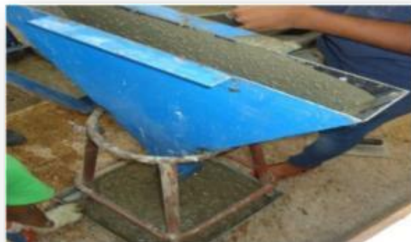
Figure 5: Test carried out in V-Funnel
